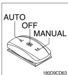
(1) This switch use to control the cooling fan.
