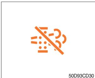
① This warning lamp lights ON when the exhaust system cleaning switch is pushed inhibit position, therefore automatic and manual exhaust system cleaning can not occur. It should inhibited, before caused fire due to the exhaust gas in high temperature.
