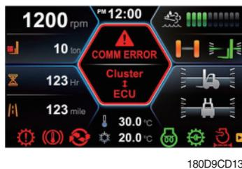
※ Main screen when occurred communication error between the cluster and TCU/ MCU / ECU
