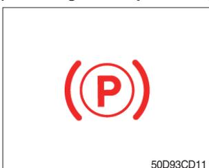
① When the parking brake is actuated, the lamp lights ON.
