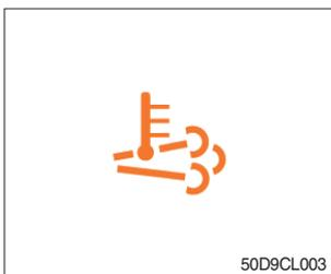
① This warning lamp indicates, when illuminated, that exhaust temperatures are high due to exhaust system cleaning.
